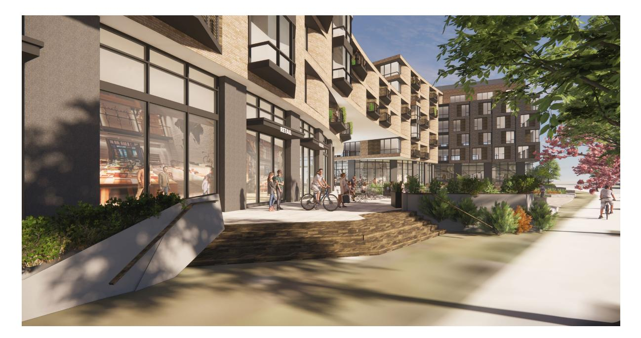
VIEW 11: Ground-level view of the entry stair and ramp into the dining terrace and generous retail landing. Sidewalk is given 8-10 additional feet of relief to create a generous welcome moment from the Pedestrian Bridge and South Water street footraffic.
